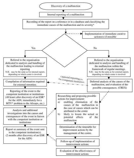
Flowchart of the procedure for handling a malfunction
